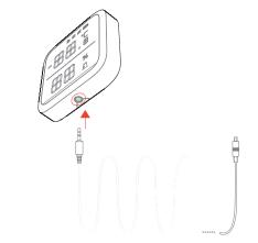
Note: The humidity detection will be disabled when using probe.
